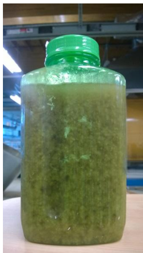
Figure 10.1. Siloxane grafting without PWCP.
