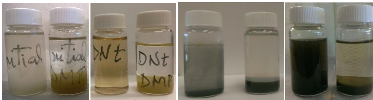
Figure 2. Vials containing field samples before (left vial) and after plasma treatment (right vial). Samples from left to right: municipal WWTP, paper mill, food processing, and anaerobic digester effluent from dairy operations.
